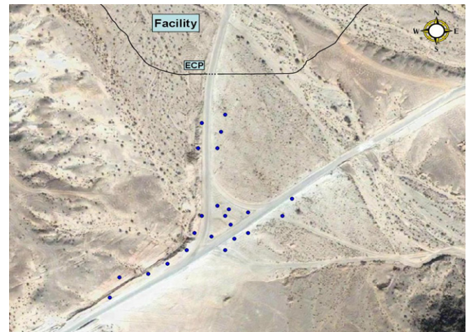
Fig. 2. Vehicle tracking scenario map. The dots represent seismic/acoustic sensor nodes. The speed, heading, location, and vehicle type are estimated by independent CARTMAP networks using binary data from all sensor nodes as input.
