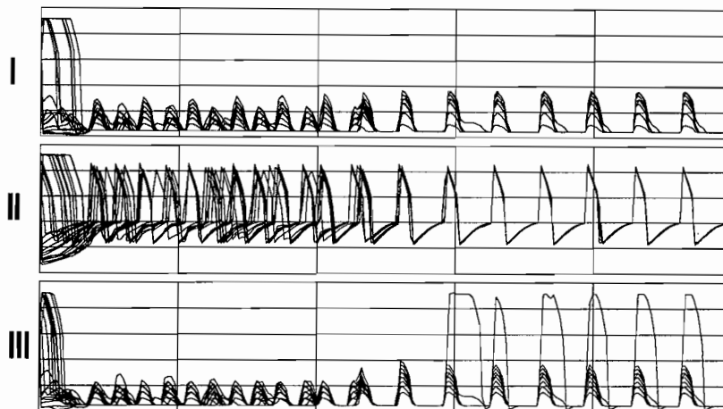
FIGURE 13. Random coupling for single bar input. Coherent oscillations rapidly emerged at positions along the bar stimulus for a random coupling shown here with \alpha = 0.1 . Each X_i provided input to six other units, chosen randomly. These random connections remained fixed throughout the simulation. Since connections were random some units received input from more than six units while others received less. In window III oscillatory activity is induced in one unit which received more than six inputs. All other background units exhibited only subthreshold oscillations.
