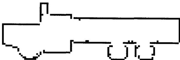
FIGURE 14. Computer simulation of CORT-X filter output  $B(x)$ .
