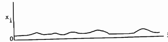
Figure 4b. Noise Contamination: Suppose that the inputs I_i have small overall intensity because I \approx 0 . Suppose also that the cells v_i are perturbed by small noisy inputs, either due to their interval metabolism or to extraneous inputs. Then the cell activities x_i can register both the inputs and the noise. The relative intensities \theta_i are consequently not accurately registered in the relative sizes of the x_i .
