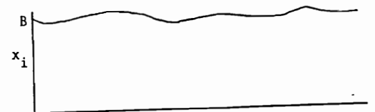
Figure 4c. Saturation: Suppose that the inputs I_i have large overall intensity because I \gg 0 . Since each cell v_i has only B sites, even the smallest input I_i may be large enough to turn on essentially all the sites of v_i if \theta_i > 0 . Then all the activities x_i will approximately equal B . Again the relative activities \theta_i are not accurately registered by the x_i . The x_i are "insensitive" to the ratios \theta_i because each of them has saturated at B .
