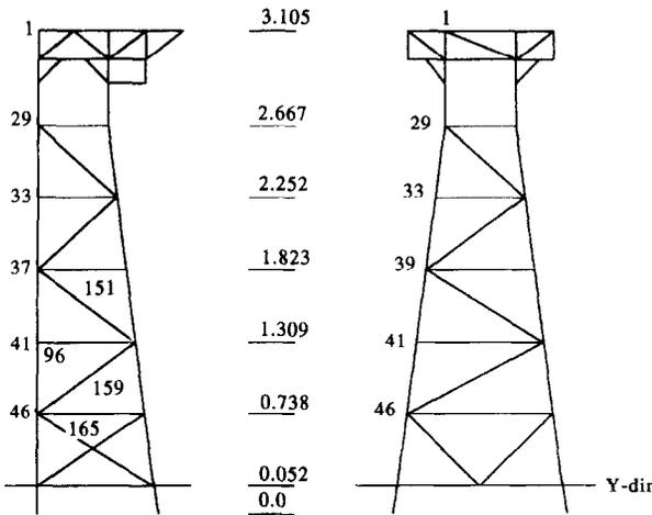
Fig. 4. Different views of the jacket platform model.
