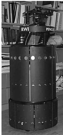
Fig. 7. The RWI B21 mobile robot employed in the experiments.
