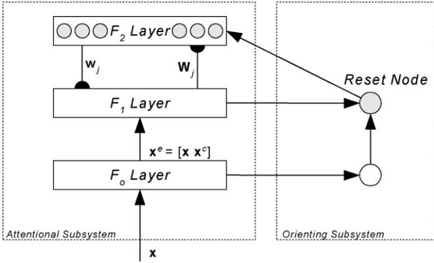
Fig. 1. Block diagram of a Fuzzy-ART module.
