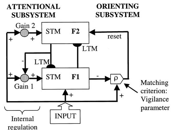
Fig. 1. Architecture of the ART1 network. The short-term memory (STM) patterns are stored in F1 and F2 layers. The long-term memory (LTM) of the system is represented by the adaptive weights of both bottom-up and top-down connections. Excitatory paths are denoted by a plus sign; inhibitory paths are denoted by a minus sign.
