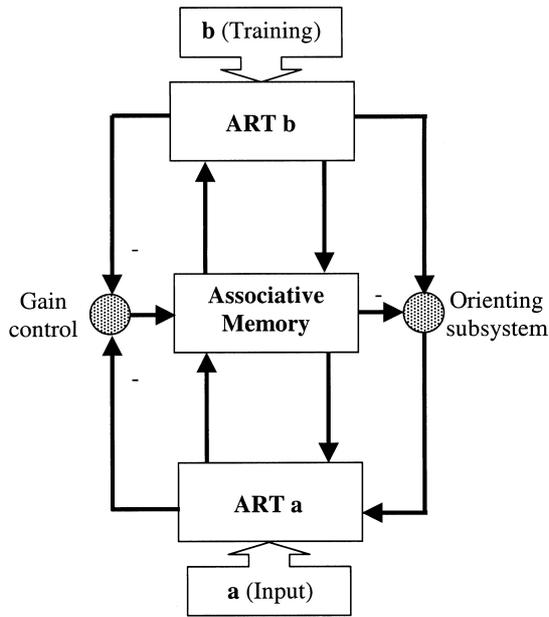
Fig. 2. Architecture of the Fuzzy ARTMAP network. It consists basically of two ART modules interconnected by an associative memory (or map field) and some internal control structures that regulate learning and information flow. Inhibitory paths are denoted by a minus sign; other paths are excitatory.
