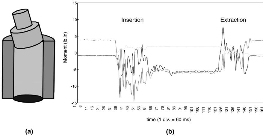
Fig. 2. (a) Peg-in-hole insertion and (b) contact force.
