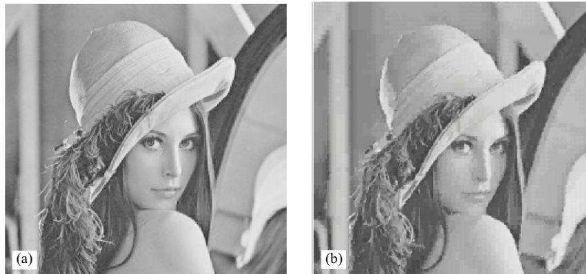
Fig. 3. (a) The original “Lena” image and (b) the reconstructed image (0.5 bpp) by CNN-ART, PSNR = 29.951 dB.
